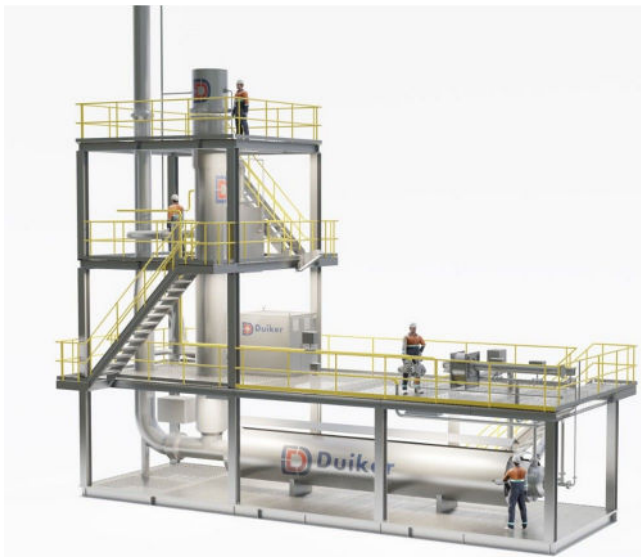
3D model of the AMMONEX pilot plant. Critical test elements match the full-scale unit.
